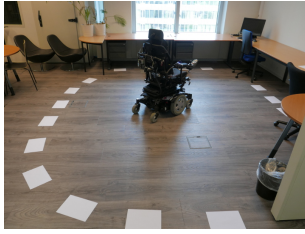
Fig. 1. Left: our motorized wheelchair in a 4-by-4 meters area. Right: BDPI is the only algorithm able to learn to avoid obstacles in 2 hours, and even outperforms a good human-designed policy. Our demonstration is a slightly more challenging task, as obstacles will be people, and the agent will be able to clear its throat to try to get people to make way for it.
