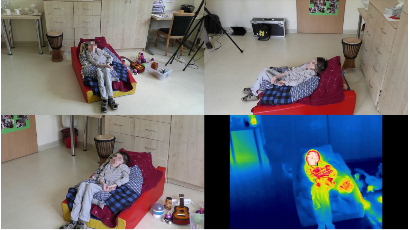
Figure 1: An example of the videos recorded. Computer vision algorithms are ran on all the streams and the results collated based on probability.
