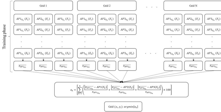
Fig. 1. Proposed mean-offset algorithm
