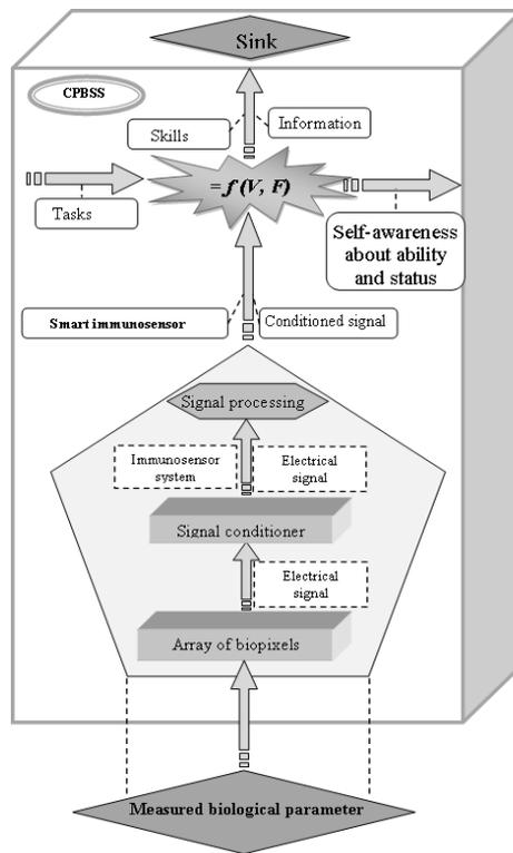
**Fig. 1.** Functional scheme of CPBSS.
