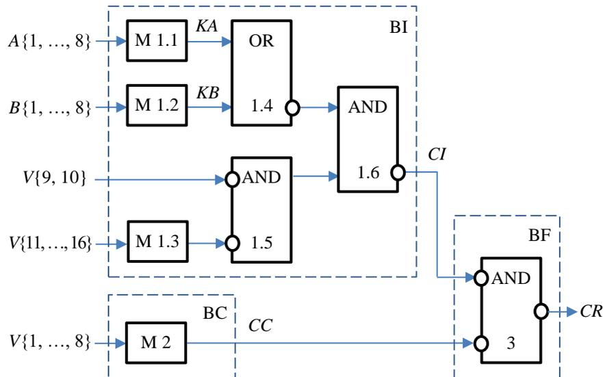
**Fig. 2.** Circuit of error detection in iterative array multiplier.
