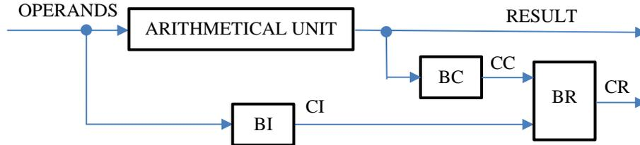
**Fig. 1.** Circuit of error detection.
