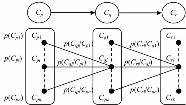
**Fig. 5.** The scheme of total probability calculation for a linear connection between chance nodes.
