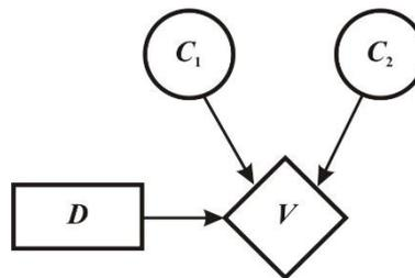
**Fig. 2.** Minimal influence diagram with two chance nodes  $C_1$  and  $C_2$ .
