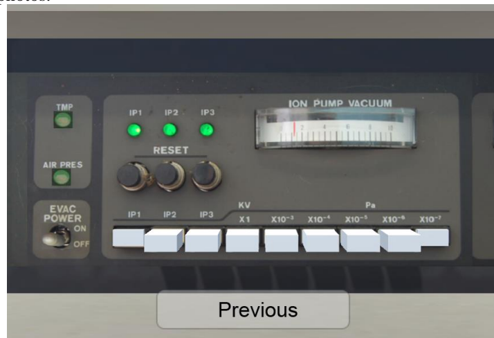
Fig. 4. Checking the vacuum level in three microscope chambers.
