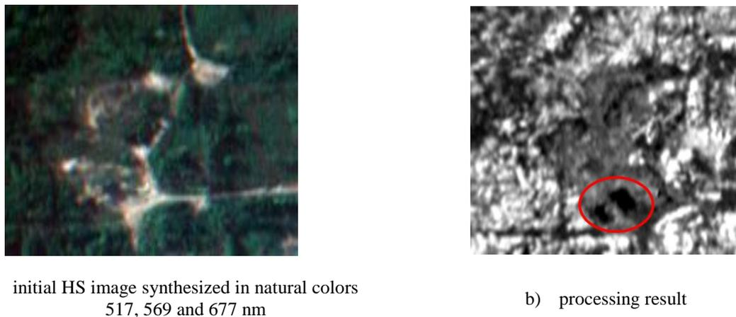
**Figure 4.** HS data –based detection of petroleum contaminated soil.
