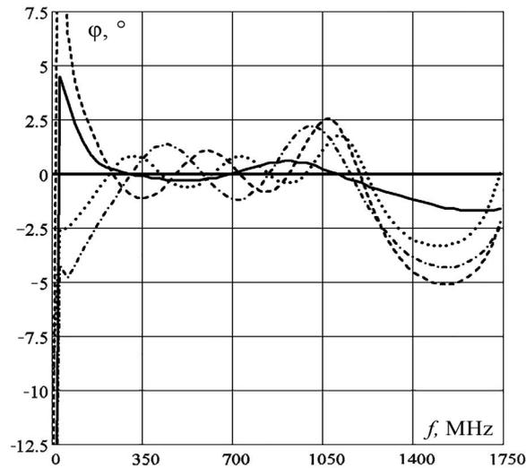
Fig. 3. Dependence of absolute errors of direction finding on the frequency of a signal without a carrier: solid line – 0°, dotted – 10°, dashed – 20°, dashed-dotted – 30°, fine line – 40°.
