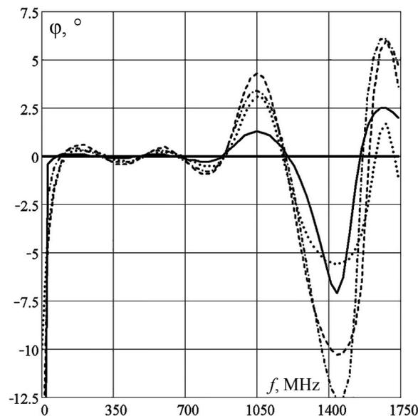
**Fig. 4.** Dependence of absolute errors of direction finding on the frequency of the signal with the carrier: solid line – 0°, dotted – 10°, dashed – 20°, dashed-dotted – 30°, fine line – 40°.
