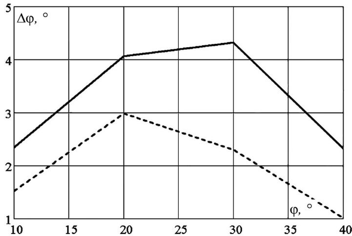
**Fig. 7.** Dependence of the root-mean-square error of direction finding from the azimuth of the arrival of the signal: solid line – on carrier, dashed line – free space.
