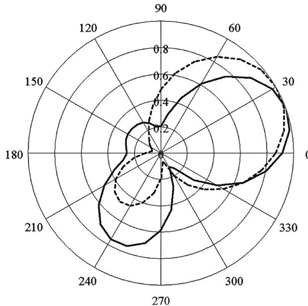
**Fig. 5.** The radiation patterns for the angle of arrival of the wave  $30^\circ$  and frequency 1450 MHz: solid line – free space, dashed line – on carrier.
