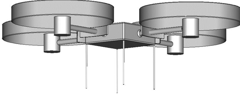
Fig. 2. 4-element antenna array and carrier.
