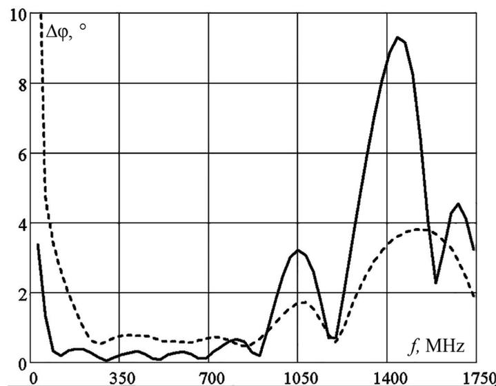
**Fig. 6.** Dependence of the root-mean-square error of bearing detection on the frequency of the signal: solid line – on carrier, dashed line – free space.
