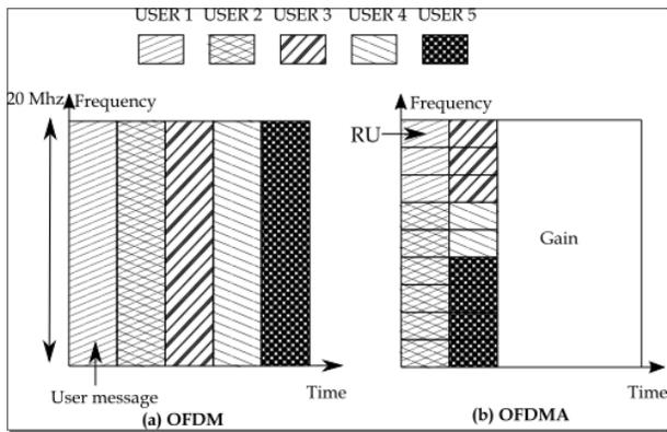
Fig. 2. Configuration of RUs on a 20 MHz band
