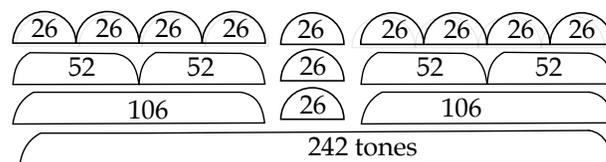
Fig. 1. Configuration of RUs on a 20 MHz band [2].
