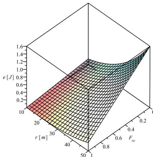
Fig. 5: Dependence of energy consumption on radius of small circle and probability of movement of sensor devices.
