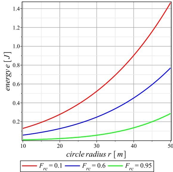
Fig. 6: Dependence of energy consumption on radius of small circle for different values of probability of movement of sensor devices.
