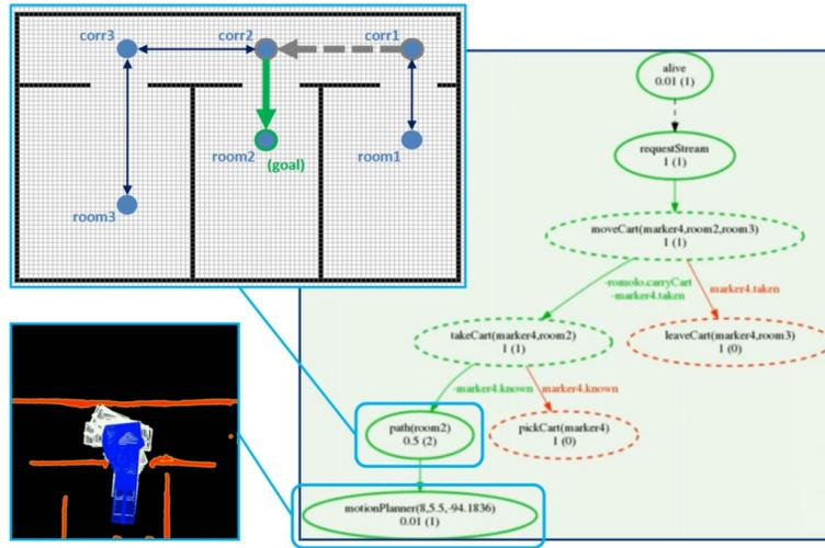
**Fig. 2.** A hierarchical task that invokes path and motion planning processes. Combined task, path, and motion planning can be also invoked.
