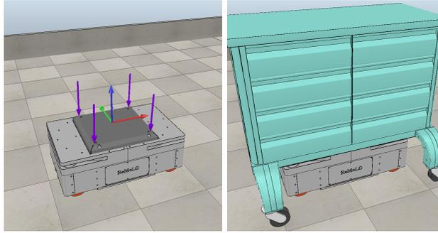
**Fig. 3.** Mobile robot carrying (right) and not carrying (left) a cart. Arrows represent the load cells used to weigh the cart (purple arrows) and to estimate external torque (around blue arrow) and forces (red and green arrows).
