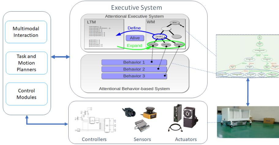
**Fig. 1.** The system architecture of RoMoLO. The executive control system orchestrates hierarchically decomposed tasks. It implements an supervisory attentional system that regulates the execution of multiple tasks allocated as hierarchical behaviors. Specialized modules are deployed to enable human-robot interaction, task and motion planning, low-level control.
