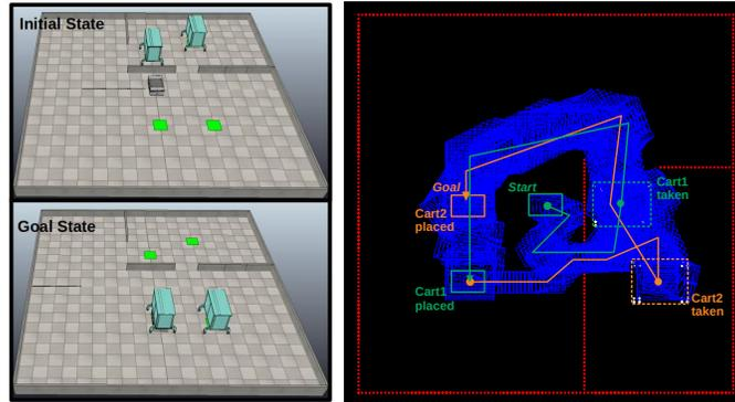
**Fig. 6.** Integrated task and motion planning for a two cart scenario: the robot is to move both carts (top left) outside the room (bottom left). In the generated plan (right) blue rectangles represent samples of the robot plan.
