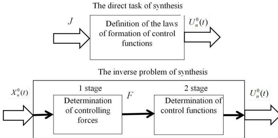
Fig. 5. Block diagram of the synthesis problem statement
