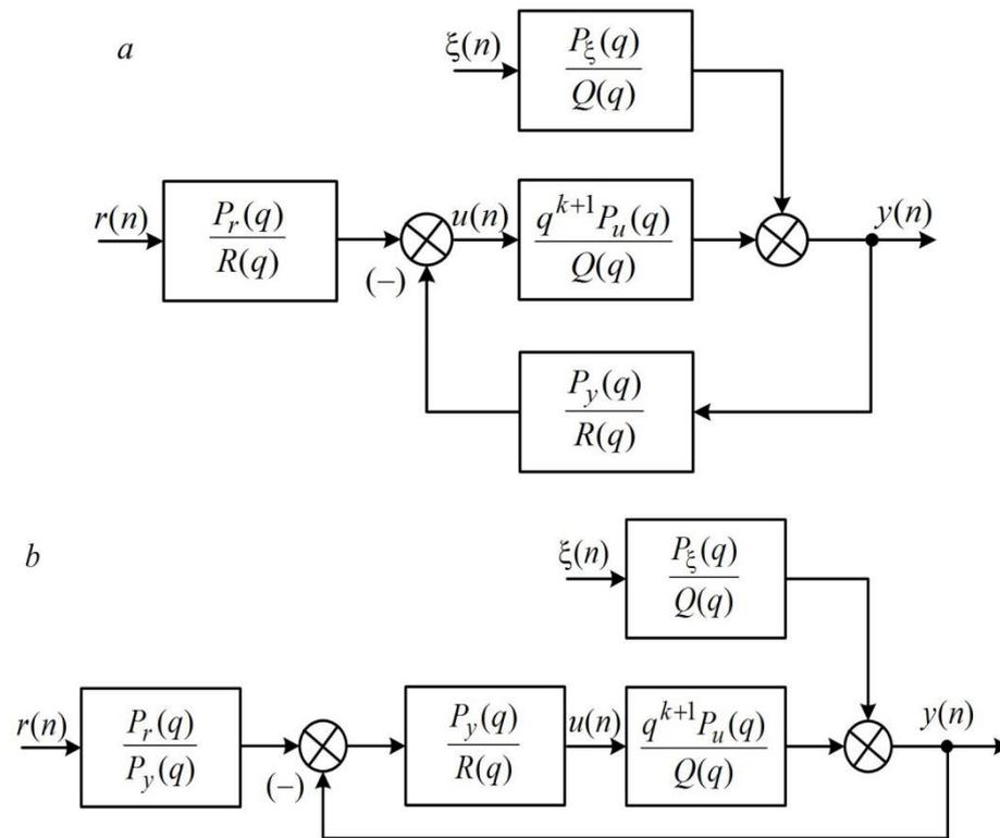
**Fig. 3.** Structural (a) and equivalent (b) schemes of a closed system
