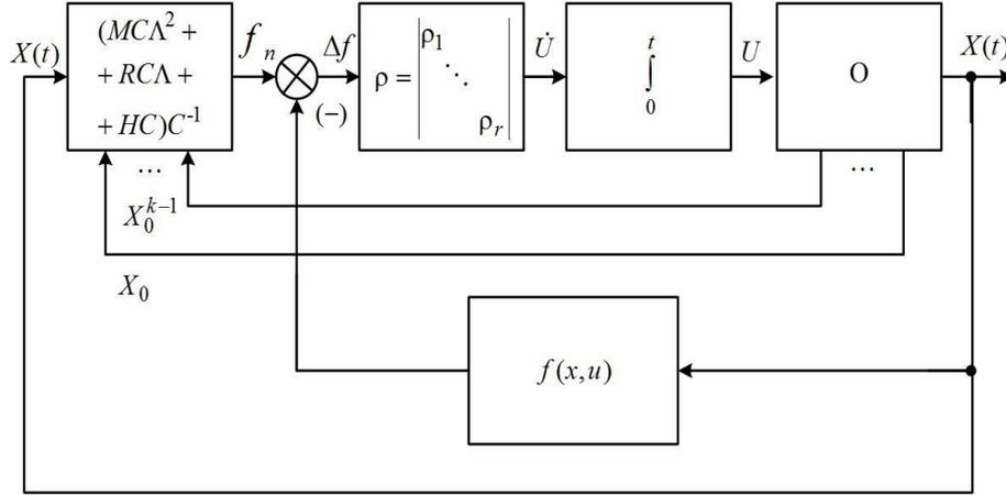
**Fig. 7.** Structural diagram of functionally stable control system by the method of inverse dynamic problems
