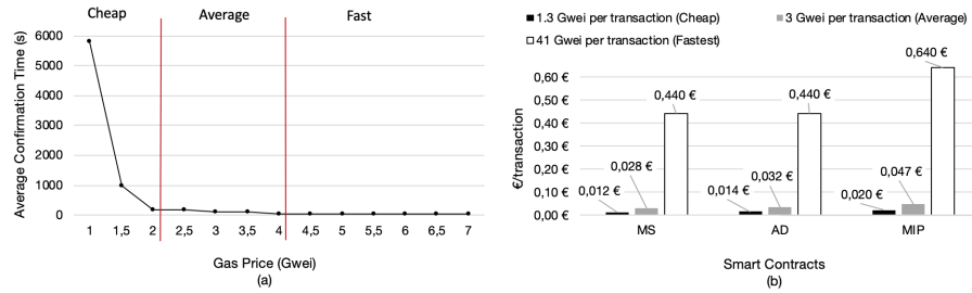
Fig. 3. Gas value required to execute all the functions of the smart contracts generated for each service in the considered case study.
