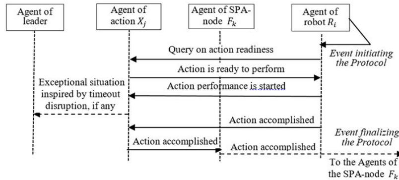
**Figure 5:** Sequence diagram of the group control Protocol – interaction of the related agents
