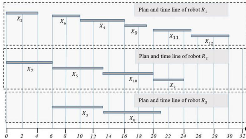
**Figure 6:** Gant diagram representing allocation of robots over the scenario actions and time line of assembly operation performance
