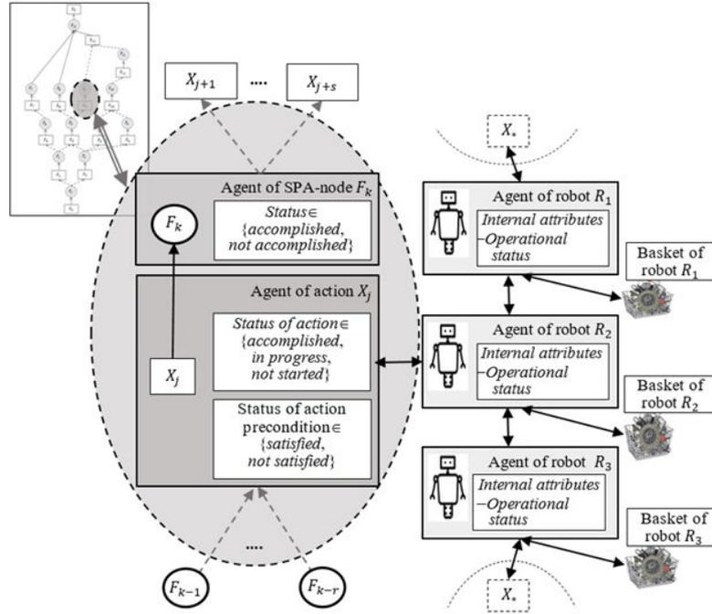
**Figure 4:** Local formal model of autonomous group control of robotic assembly process: agents, state machines, attributes of state machines, and their interactions
