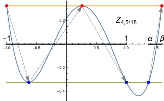
Figure 1: The equioscillation property of  $Z_{4,5/18}^*$ .
