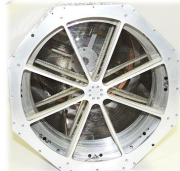
Fig. 4. Front view of the dust impact dust particle sensor: the grid, the target of the device and the particle detector input window.
