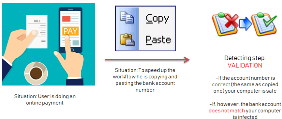
Figure 2: Sample attack detection scheme in which the information is analyzed by comparing it to background data pattern.
