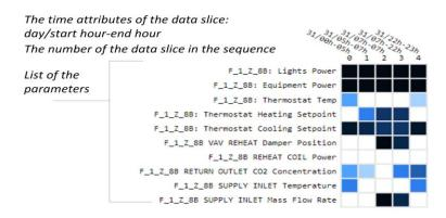
Fig. 2. The matrix-based presentation of the HVAC data
