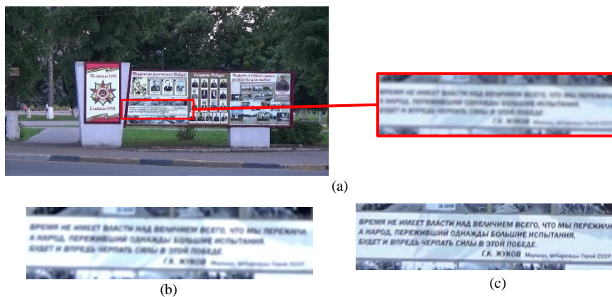
Fig. 3. An example of restoration based on the average gradient of a photo of a commemorative inscription on a stand in Lenin Public Gardens, Bryansk: a) the original segment, b) restoration by maximizing the average gradient, c) the best option, selected manually.
