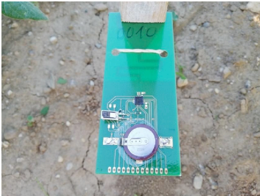
Fig. 2. Smart badge with microchip, sensors, antenna and battery button.
