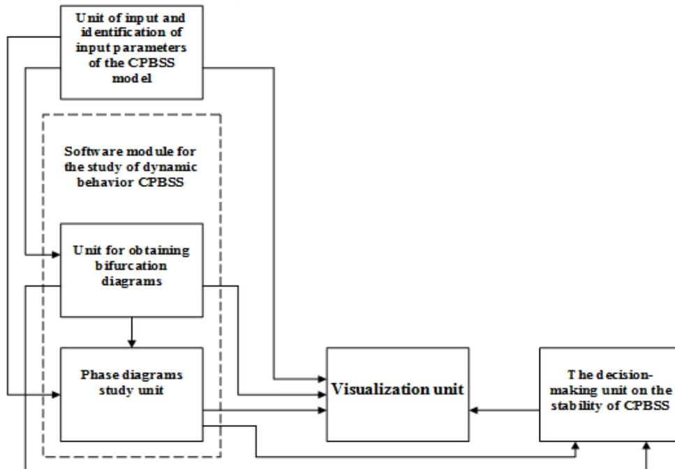
**Figure 6:** Block diagram of the software package for the study of phase diagrams CPBSS
