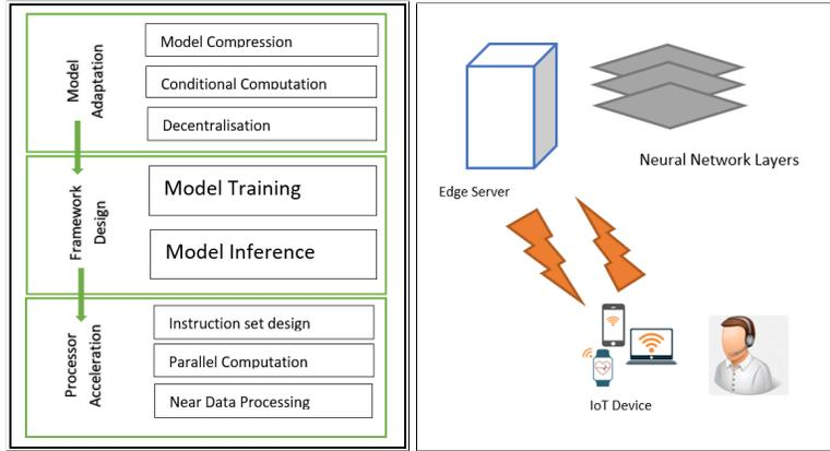
**Fig. 1.** A road map of edge intelligence on a top-down decomposition [10](left). Edge Computing structure for IoT Devices(right)
