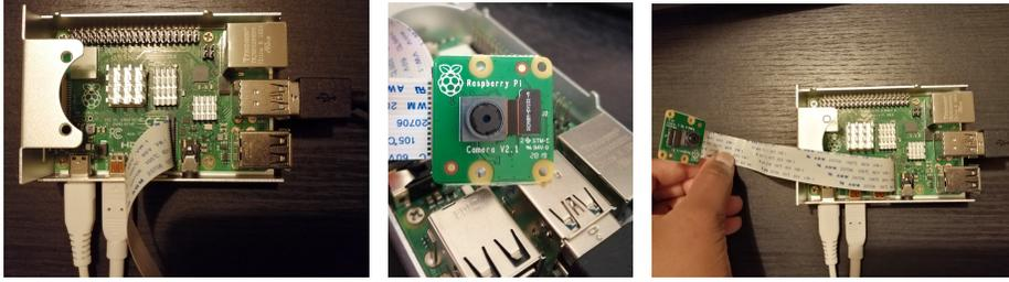
**Fig. 2.** A picture of the edge computing experiment setup used in this paper. Extreme-left is a Raspberry Pi 4 Module, center is a Pi camera module and the extreme-right image shows the connection of Pi camera on the Raspberry Pi Module. The USB ports helps connect the mouse and keyboard for control and the display device is connected to the HDMI port.
