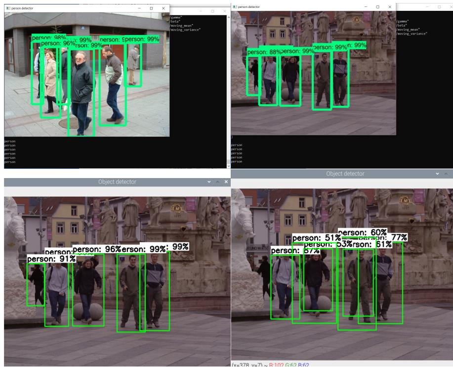
**Fig. 4.** The top two images show person detection from the INRIA dataset using unquantized SSD MobileNet Model. The bottom row of pictures show detections from the Raspberry Pi. The bottom-left image is a fully accurate detection comparable to the GPU and the bottom-right is an image with two False-Positives
