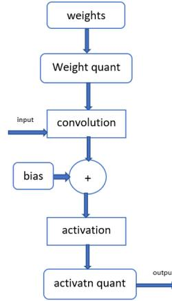
**Fig. 3.** The flow-diagram of training with simulated quantization [15]
