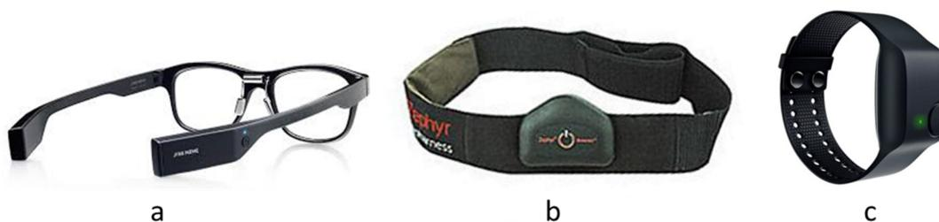
**Figure 1.**Wearable devices. a) J!NS MEME ES\_R glasses, b) Zephyr Bioharness 3.0 chest strap, c) Empatica E4 wristband.
