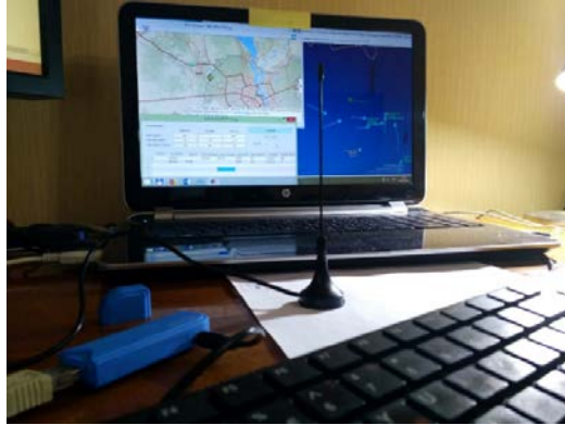
Fig. 3. SDR and software for data decoding
