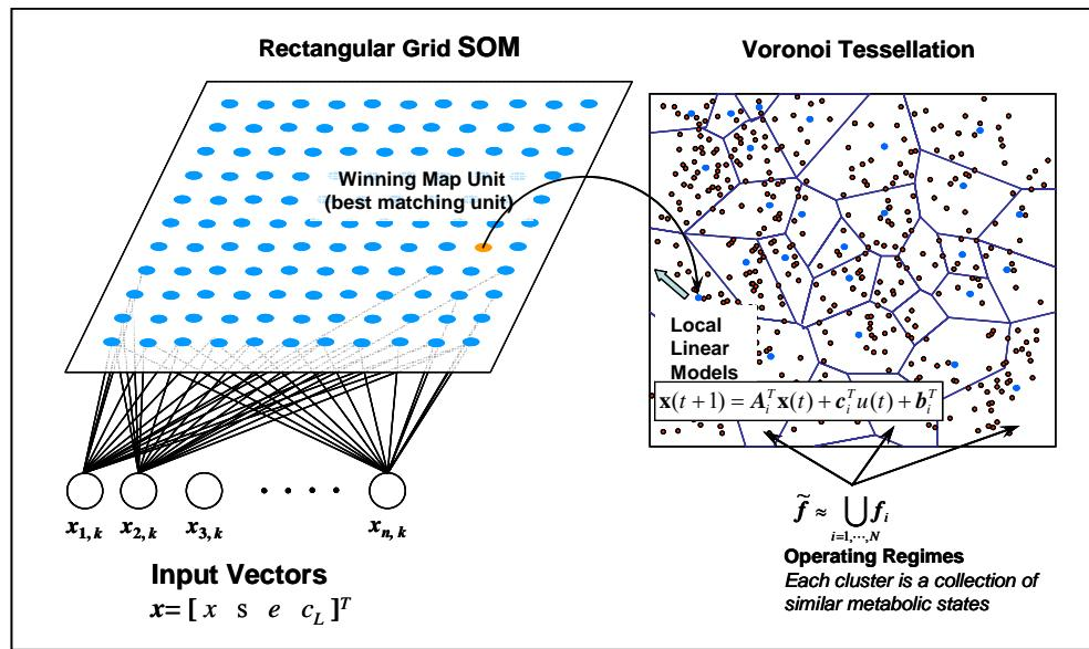
**Fig. 1** Representation of the SOM based local linear model of the ethanol fermentation process
