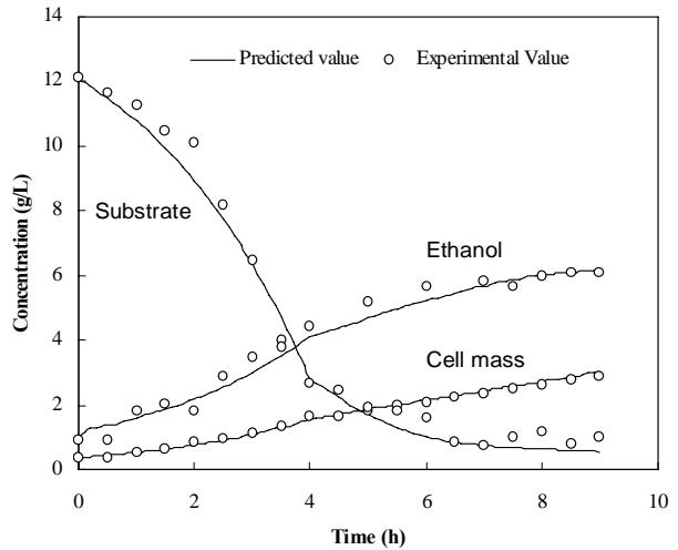
**Fig. 4 On-line control implementation of SOM-MLLM feed forward controller for *S. cerevisiae* fermentation process in a 15 L reactor. The desired trajectory is to control the cell mass concentration along the profile  $x = 0.3 \times \text{time}$**
