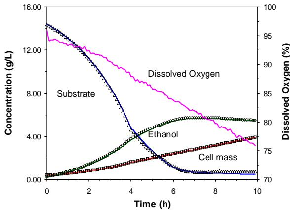
**Fig. 3 A comparison of the prediction of the SOM-MLLM during recall. The result for initial condition III is shown here. — Simulated from the model. All symbols are prediction of SOM-MLLM ( $\Delta$  substrate  $\circ$  ethanol  $\square$  cell mass)**
