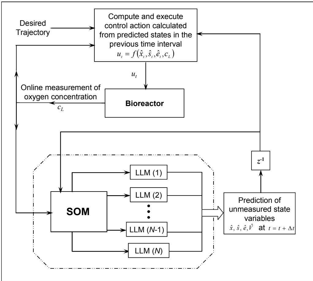
**Fig. 2 Block diagram for application of SOM based models to control yeast fermentation by using a feed forward control law**
