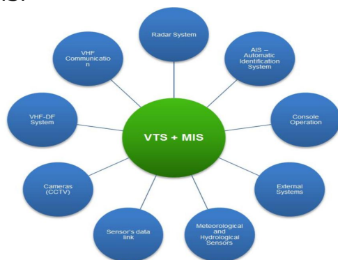
Fig.1.Schematic diagram of the input and output components and subsystems of a VTMIS [24]
