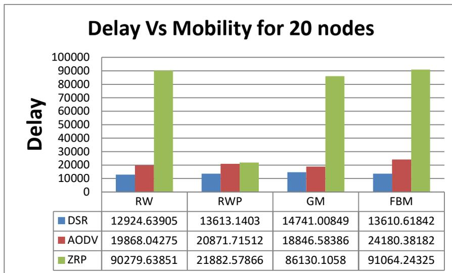
**Figure 7:** Delay versus mobility model for 20 nodes.
