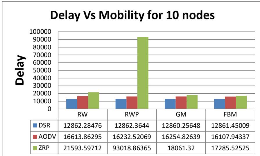
**Figure 5:** Delay versus mobility model for 10 nodes
