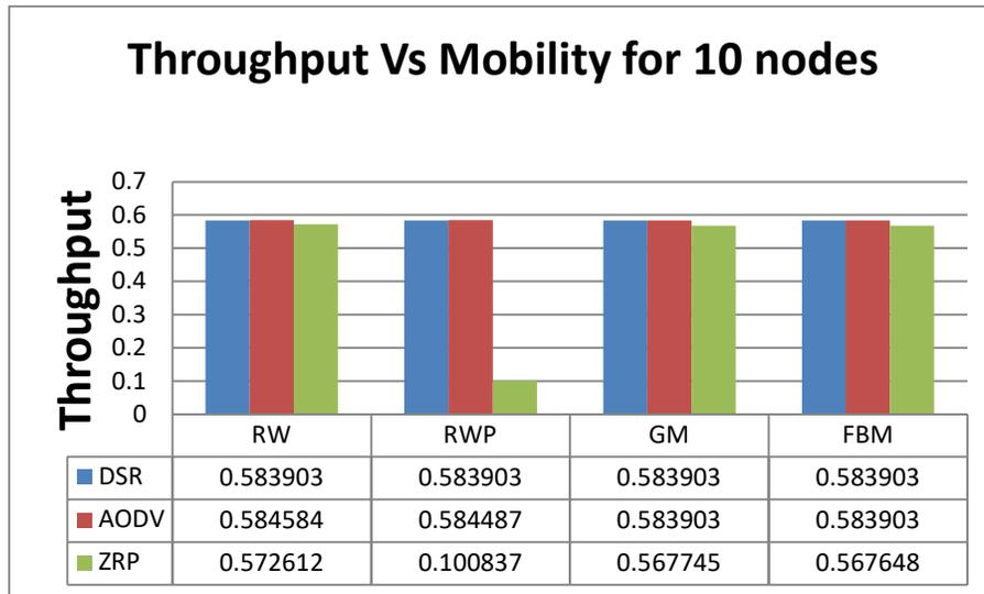
**Figure 4:** Throughput versus mobility model for 10 nodes.
