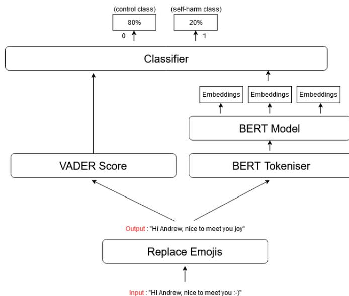
**Figure 6:** Pipeline of the third model proposed.
