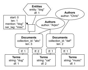
**Figure 7:** Example property graph for the TREC News Track's background linking task. The node types are authors, entities, terms and documents. Edges connect document nodes to other types of nodes. Both edges and nodes can have properties (following the property graph model). Multiple edges may exist between one entity node and one document node, as one entity can be linked multiple times to one document.
