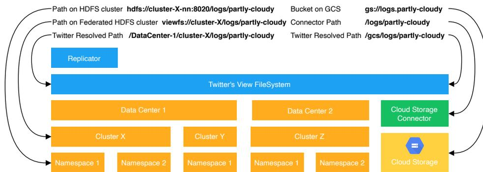
Figure 6: Architectural design of the storage federation.
