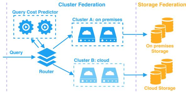
**Figure 3:** Architectural design of the cluster federation.
