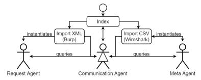
**Fig. 1.** Overview of the prototype. The workflow starts at index.jsp. By importing a Wireshark or Burp Export, the corresponding agent will be initialized. Afterwards, the user may send queries to the communication agent.
