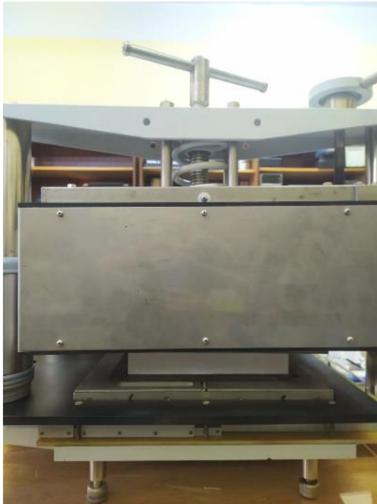
Figure 1: Heat module of the system during sample installation
