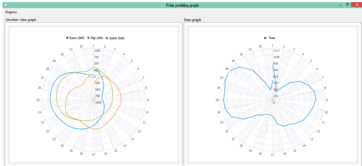
Figure 7: a) Polar graph of the k.h.a. joints power b) Polar plot of joint power sum
