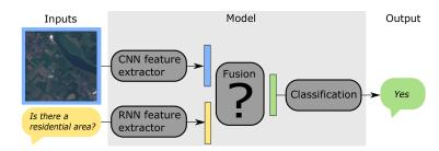
Fig. 1. Simplified representation of a VQA model for remote sensing.
