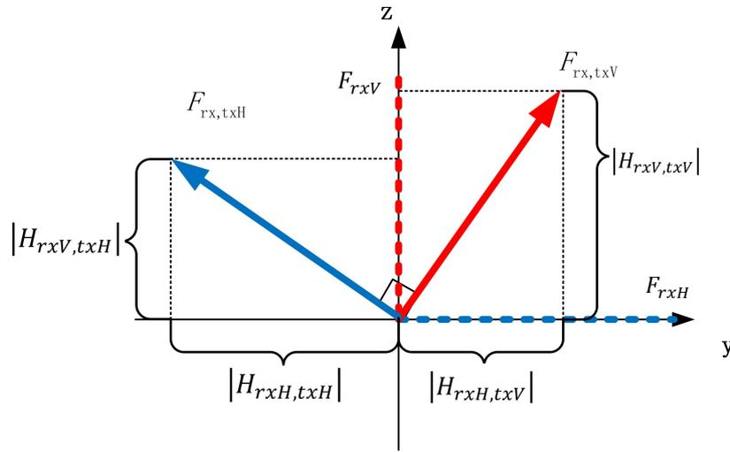
**Figure 2:** Received signals field projections on the UE Local Coordinate System.
