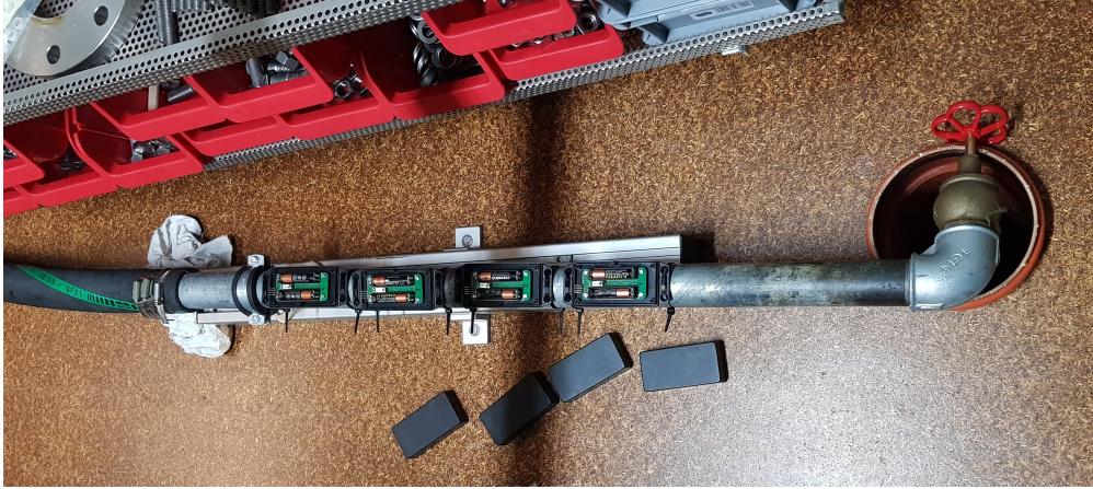
Figure 3: Experimental setup for vibration data acquisition.
