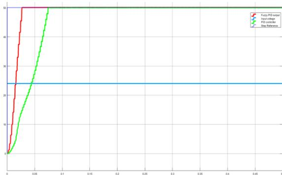
**Figure 6:** Output response (35Ω with 24V supply)
