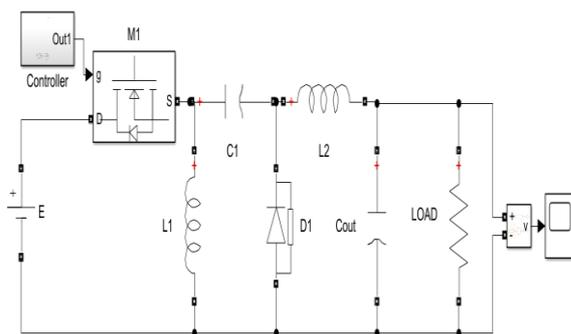
**Figure 1:** Simulink model of the ZETA converter
