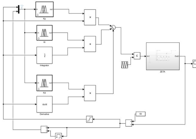
**Figure 5:** TS-ATFPIF controller for ZETA
