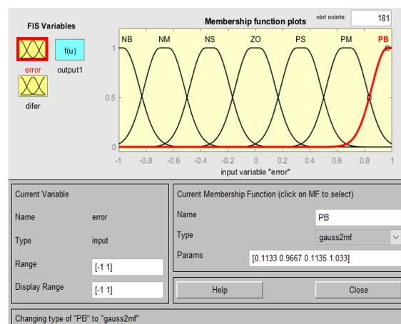
Figure 3: Membership functions for the error
