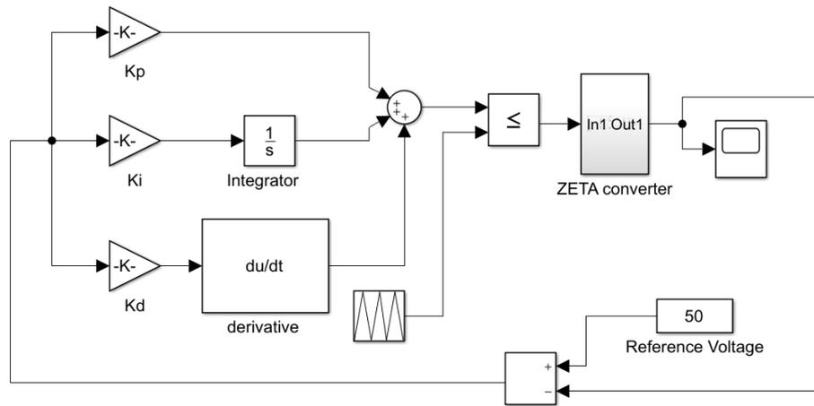
Figure 2: Simulink model of PID controller
