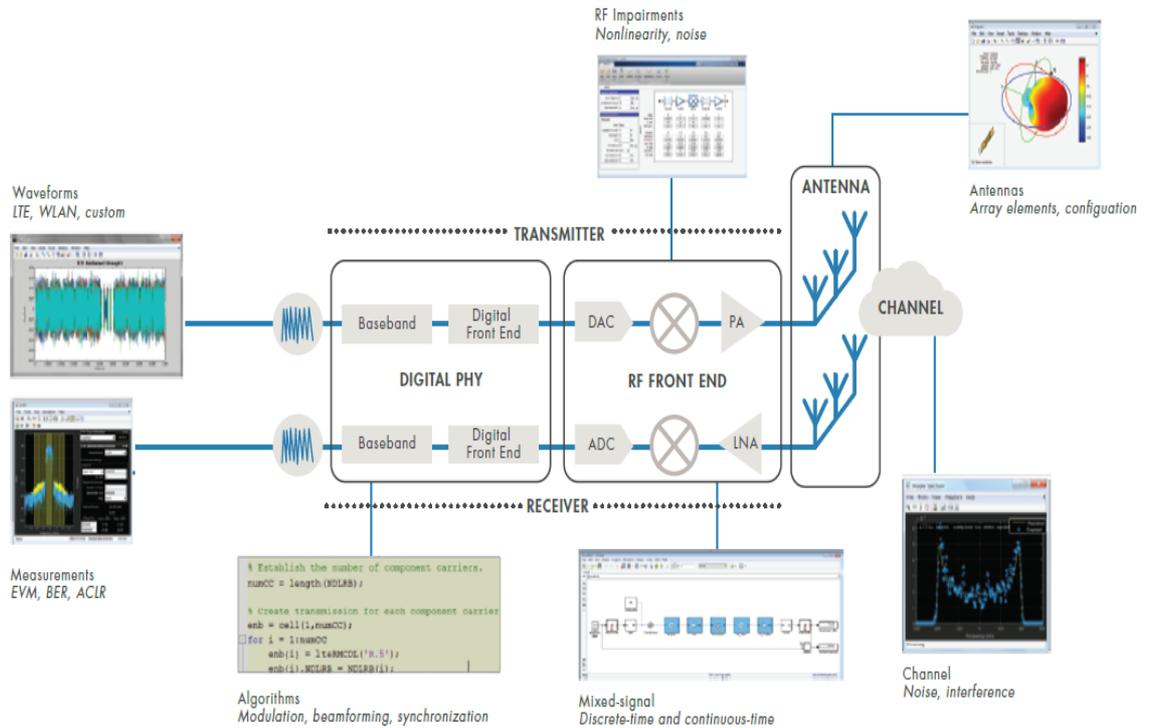
**Figure 1:** Examples of 5G Requirements and design steps
