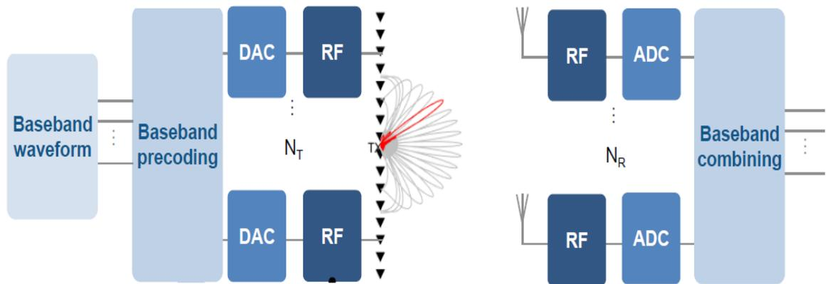
**Figure 2:** SDR and conversion from RF-baseband and vice versa
