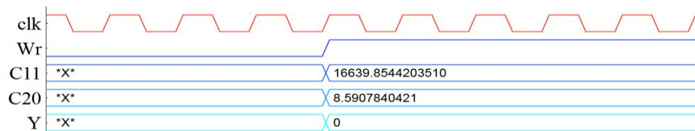
**Figure 9:** Simulation behavior of proposed NVG-RAM detector when  $w_r$  input signal is activated
