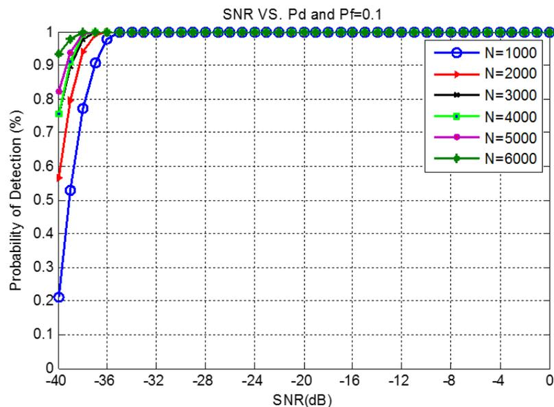
Figure 5: SNR versus Pd, for NVGRAM
