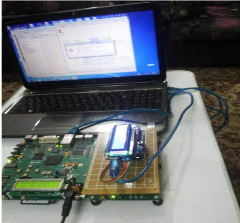
**Figure 8:** Spartan-3A DSP board and Arduino Uno Connection
