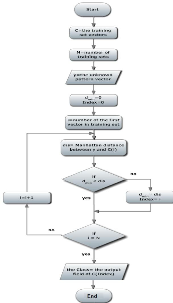
Figure 3: Flowchart of recall phase of NVG-RAM
