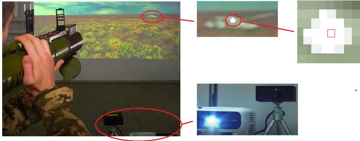
Figure 1: Multimedia weapon simulator with a laser emitter.
