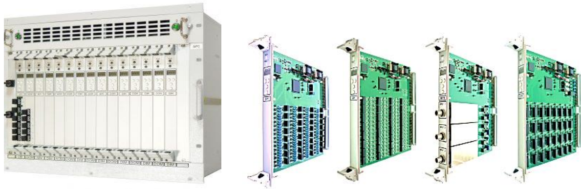
Figure 2: FPGA-based platform RadICS and its modules
