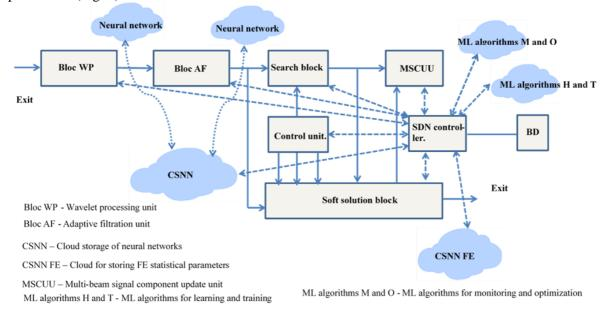
**Figure 1:** Block diagram of the proposed architecture of the receiving system of the THz band using algorithms based on artificial intelligence
