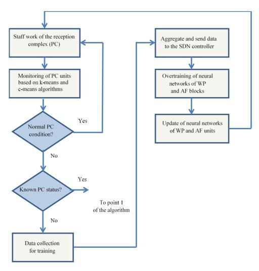
**Figure 5**: Block diagram of the algorithm for tracking the state of the receiving complex for the collection and retraining of the corresponding neural networks
