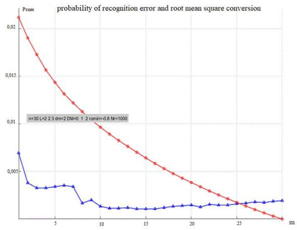
**Figure 4**: Dependences for the total probability of error and UPC transformation on the dimension of the feature vector after the transformation algorithm of the principal components
