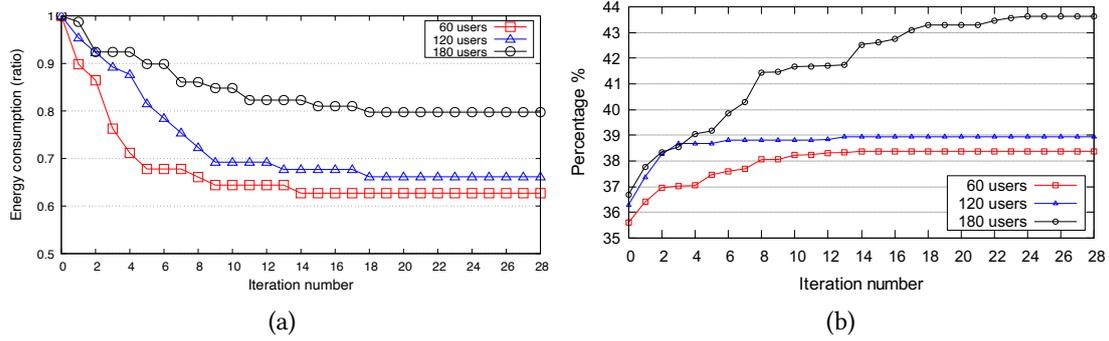
**Figure 1:** Temporal evolution of the levels of energy (a) and average latency (b)
