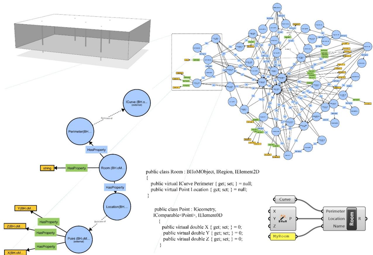
Figure 3: BHoM RDF building demonstrator, with a zoom on the Room class.
