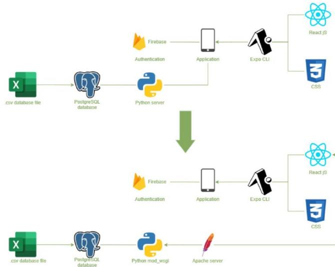
**Figure 1:** System diagram. Initial and final versions
