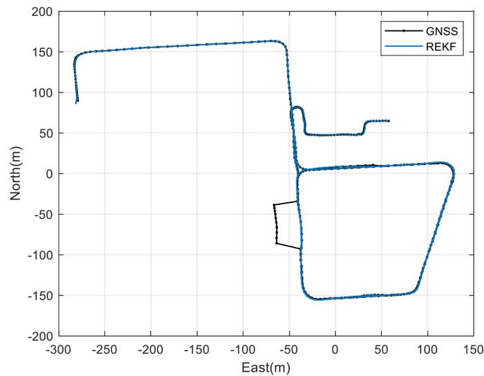
**Figure 8:** The abnormality lasts for 10s in GNSS
