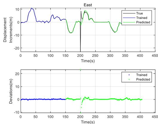
**Figure 10:** Prediction increment and deviation when the abnormality lasts for 11s
