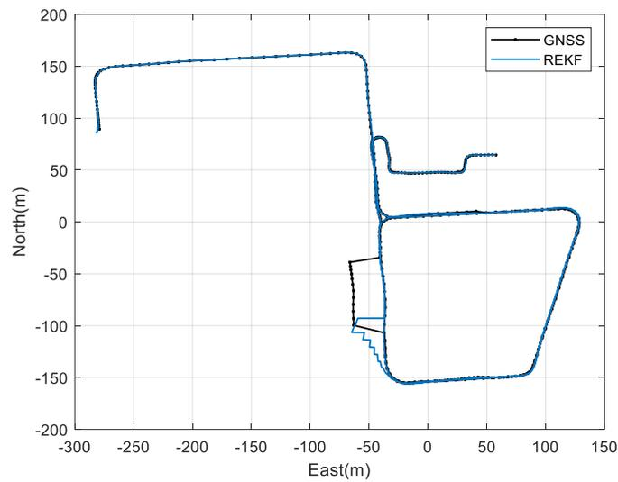
**Figure 9:** The abnormality lasts for 11s in GNSS
