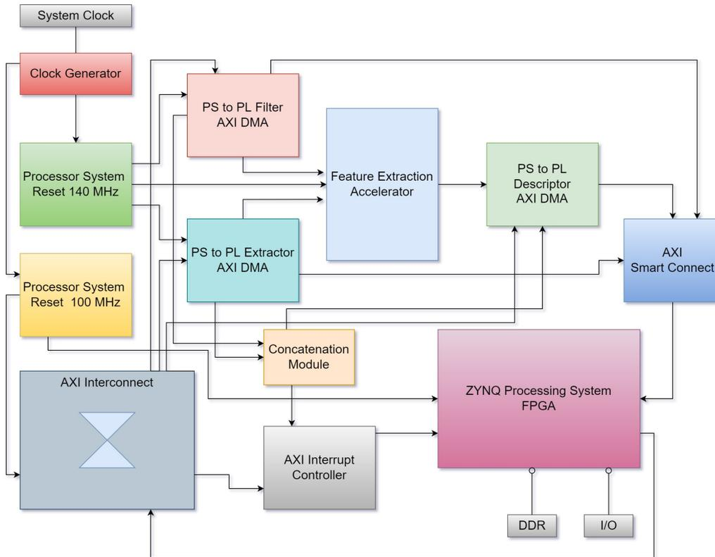
**Figure 4.** Proposed hardware accelerated ORB feature extractor
