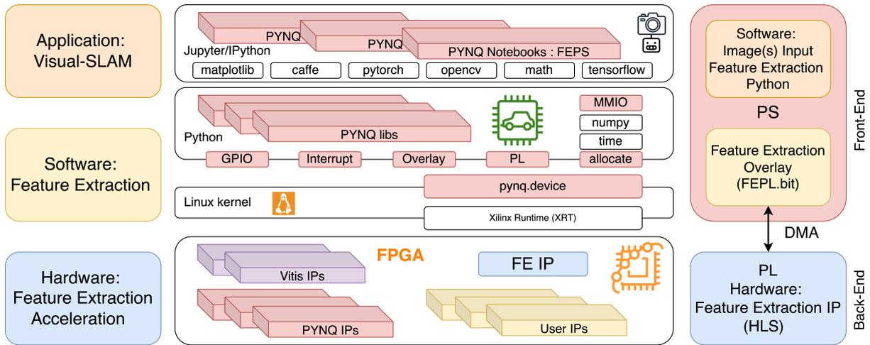
**Figure 1.** HILO co-design framework using PYNQ
