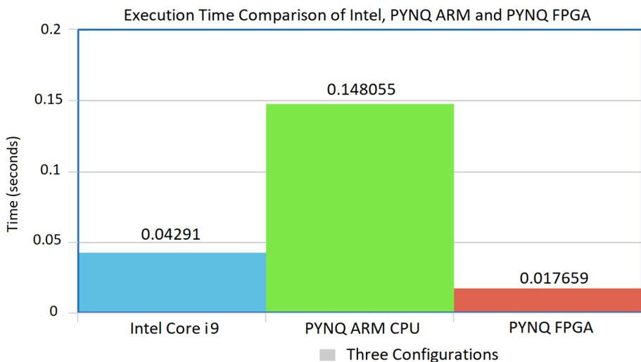
**Figure 9.** Execution Time Comparison using three platforms
