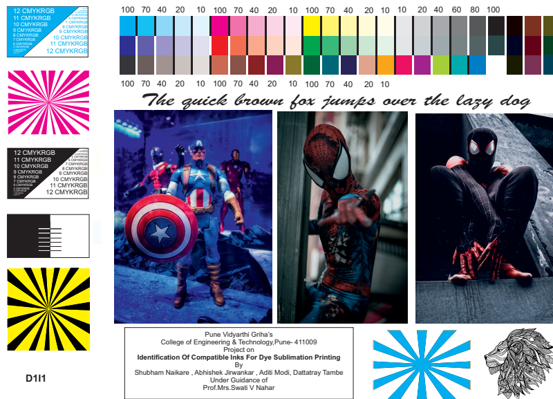
Figure 2: Test chart printed on both the substrates using the original and compatible inks
