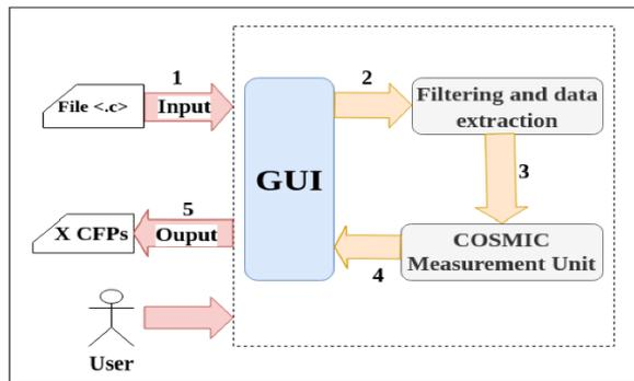
**Figure 3:** A simplified architecture of the COSMIC-C tool prototype
